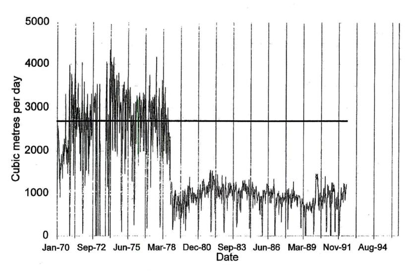
FIGURE 8: GRAPH OF ABSTRACTION FROM THE UNILEVER SITE FROM 1970 - 1993. THE HORIZONTAL LINE MARKS THE CURRENT CONSENTED DAILY TOTAL. GRAPH SOURCED FROM TONKIN & TAYLOR (1997)
